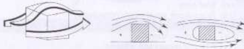
Fig. 2.10 Pressure difference caused by obstacles
